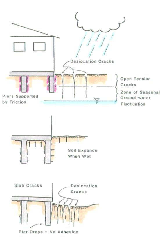
The figure above taken from *Ref. 4.0* shows how water can find its way into and under a structure. In addition several other soil mechanisms and behavior tend to cause this cyclic
