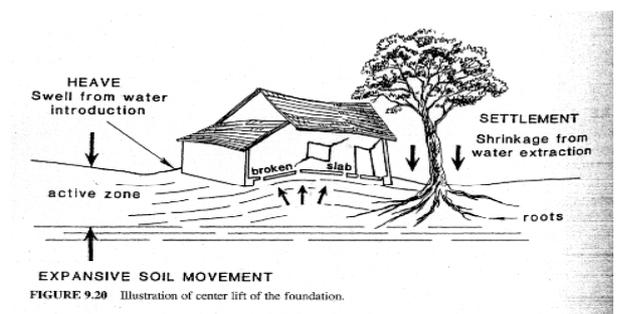
The figure above shows how Moisture variation is caused by natural processes. In addition to this, water tend to move from hotter areas to cooler areas (such as under structures) in a process known as “*Thermal Migration*”. Thus over a period of time water would be slowly injected underneath structures further aided by *Matric Suction*.
